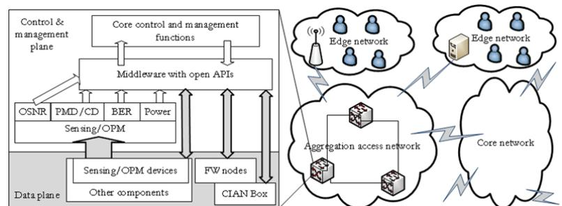
Architecture of control and management system for aggregation networks
