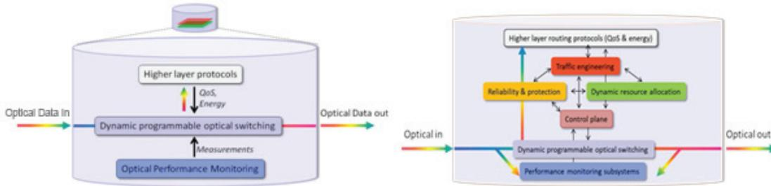
Block schematic of CIAN box (left) and detailed internal architecture (right). Higher-layer routing protocols are those that are above the physical layer in the Open Systems Interconnection stack.
