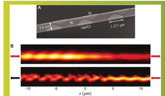
(A) Scanning electron microscope image of the fabricated device. (B) Measured near-field amplitude distribution of light in the one-way mode converter for both forward (upper) and backward (lower) light
